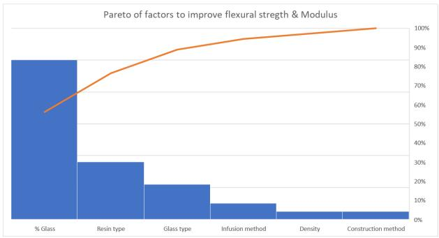
Optimizing glass percentage, resin type and glass type produces the desired performance & savings.
