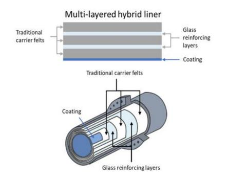
The common reinforcement layer used for relining pipes is glass. Hybrid felt is not limited to glass alone. Other fiber materials can be used to meet strength requirements for unique industrial applications.
