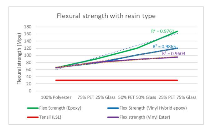
Flexural strength improved ~36% with 50% glass and vinyl ester resin. Flexural strength improved ~54% with 50% glass and vinyl hybrid resin. Flexural strength improved ~85% with 50% glass and epoxy resin.
