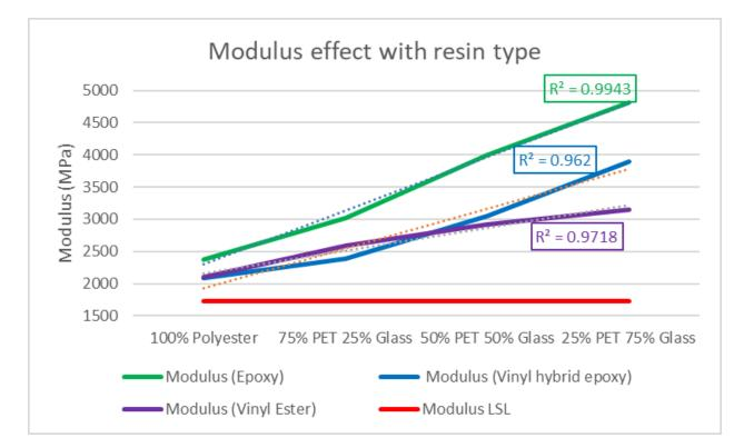
Modulus improved ~38% with 50% glass and vinyl ester resin. Modulus improved ~52% with 50% glass and vinyl hybrid resin. Modulus improved ~67% with 50% glass and epoxy resin.
